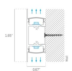
HRZ1402F is a linear profile sconce light made of extruded aluminum housing with a protective silver anodized finish, capped with a curved frosted lens.
