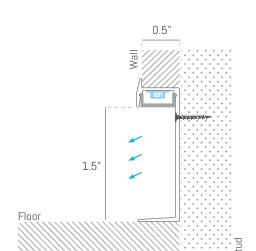
HRZ4915F is a recessed linear light made of extruded aluminum housing with a protective silver anodized finish.
