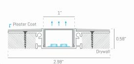
SPK7515F is a recessed linear profile made of extruded aluminum housing with a protective white sand texture powder coat matte finish, capped with a flush frosted lens.
