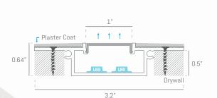
SPK8115F is a recessed linear profile made of extruded aluminum housing, capped with one inch wide flat frosted lens.
