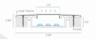
SPK8615F is a recessed linear profile made of extruded aluminum housing, capped with one and half inch wide flat frosted lens.
