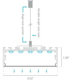
VIV10236F is a pendant linear profile made of extruded aluminum housing with a protective silver anodized finish, capped with a flush frosted lens.
