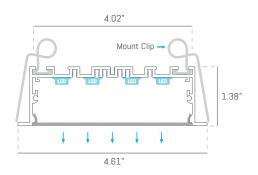
VIV11736F is a recessed linear profile made of extruded aluminum housing with a protective silver anodized finish, capped with a flush frosted lens.
