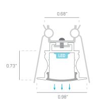
VIV1207C is a recessed linear profile made of extruded aluminum housing with a protective silver anodized finish, capped with a flat frosted lens.
