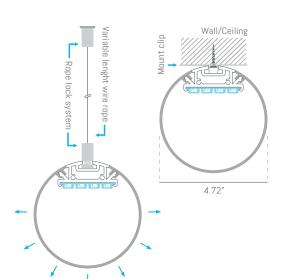
VIV120C is a pendant-surface linear profile made of extruded aluminum housing with a protective silver anodized finish, capped with a round frosted lens.
