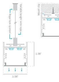
VIV3535F is a pendant-surface linear light made of extruded aluminum housing with a protective silver anodized finish, capped with a flush frosted lens.
