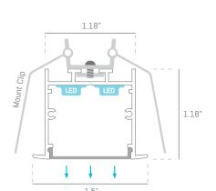
VIV3830F is a recessed linear profile made of extruded aluminum housing with a protective silver anodized finish, capped with a flush frosted lens.
