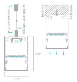
VIV4160F is a pendant linear light made of extruded aluminum housing with a protective black powder coat matte finish, capped with flush frosted lenses.
