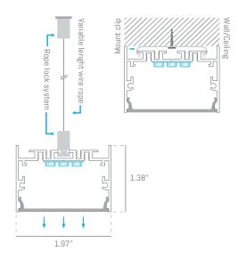
VIV5036F is a pendant-surface linear profile made of extruded aluminum housing with a protective silver anodized finish, capped with a flush frosted lens.
