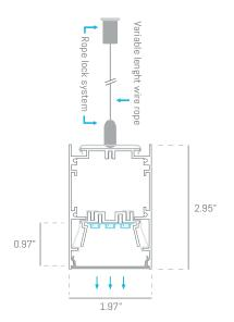
VIV5075F is a pendant linear profile made of extruded aluminum housing with a protective silver anodized finish, capped with a flush frosted lens.
