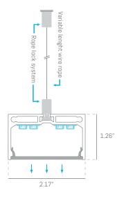
VIV5532F is a pendant linear profile made of extruded aluminum housing with a protective silver anodized finish, capped with a flush frosted lens.
