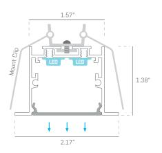
VIV5535F is a recessed linear profile made of extruded aluminum housing with a protective silver anodized finish, capped with a flush frosted lens.
