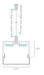
VIV5550S is a pendant linear light made of extruded aluminum housing with a protective silver anodized finish, capped with a square frosted lens that surrounds the LED housing.
