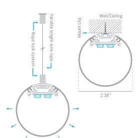
VIV60C is a pendant-surface linear profile made of extruded aluminum housing with a protective silver anodized finish, capped with a round frosted lens.
