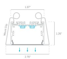
VIV6535F is a recessed linear profile made of extruded aluminum housing with a protective silver anodized finish, capped with a flush frosted lens.
