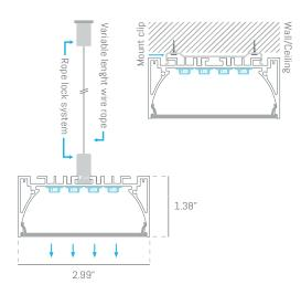
VIV7635F is a pendant-surface linear profile made of extruded aluminum housing with a protective silver anodized finish, capped with a flush frosted lens.
