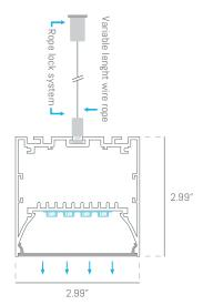
VIV7676F is a pendant linear profile made of extruded aluminum housing with a protective silver anodized finish, capped with a flush frosted lens.
