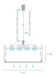
VIV8035F is a pendant linear profile made of extruded aluminum housing with a protective silver anodized finish, capped with a flush frosted lens.
