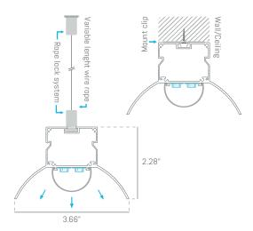
VIV9358C is a pendant-surface bay light made of extruded aluminum housing with a protective silver anodized finish, capped with a round frosted lens.
