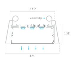
VIV9540F is a recessed linear profile made of extruded aluminum housing with a protective silver anodized finish, capped with a flush frosted lens.
