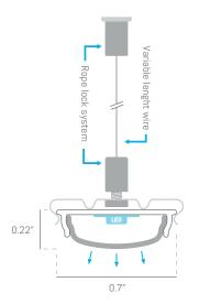
WAV1806C is a pendant-surface light made of extruded aluminum housing with a protective silver anodized finish, capped with a curved frosted lens.
