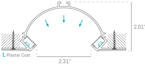
SPK13350F is a recessed linear profile made of extruded aluminum housing with a protective silver anodized finish, capped with a flush frosted lens.
