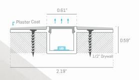
SPK5615F is a recessed linear profile made of extruded aluminum housing with a protective silver anodized finish, capped with a flush frosted lens.
