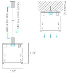
VIV3535RF is a pendant-surface linear profile made of extruded aluminum housing with a protective silver anodized finish, capped with a flexible flush frosted lens.
