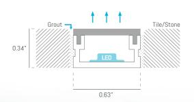
HYN1610F is a waterproof recessed surface linear profile made of extruded aluminum housing with a protective silver anodized finish, capped with a flush frosted lens.
