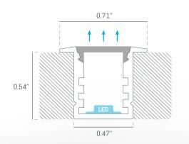
HYN1815F is a linear trim recessed profile made of extruded aluminum housing with a protective silver anodized finish, capped with a flush frosted lens.
